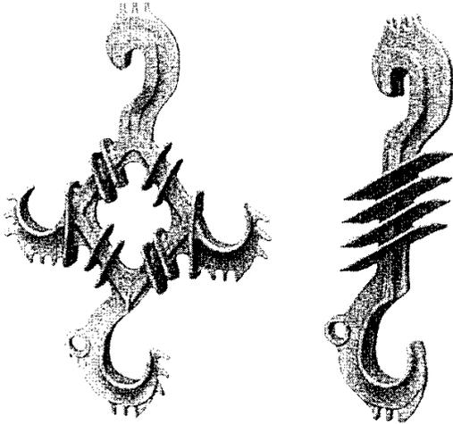
Fig. 1. Three Phase and Single Phase Spacer
